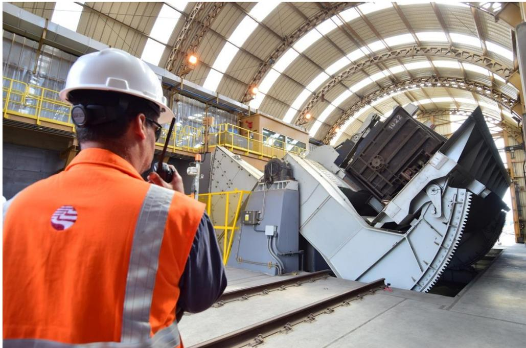
Example: SCHADE Wagon Tippler in Peru (Photo SCHADE)
