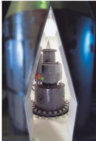
AUMUND Discharge System type CENTREX<sup>®</sup> CTX with internal drive
