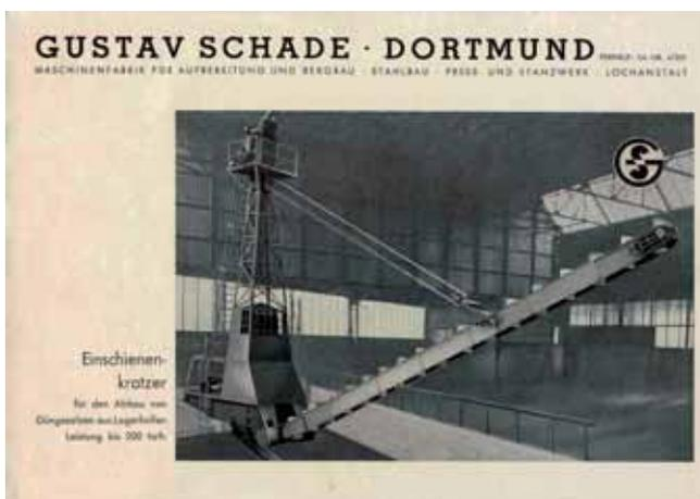
This is a single cantilevered boom design and the major elements of this machine are recognizable in today's designs but much improved in detail and construction.
