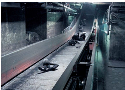
Inclined transportation of castings
